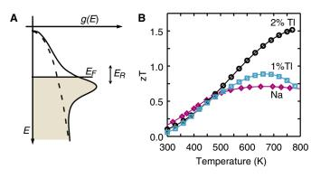
for  $Tl_{0.02}Pb_{0.98}Te$  (black squares) and  $Tl_{0.01}Pb_{0.99}Te$  (blue circles) compared to that of a reference sample of Na-PbTe (purple diamonds).
